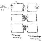
i) This test is carried out on 3-ph transformer to identify primary & secondary winding belonging to the1 Mark for same phase. circuit
